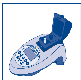
Measure initial light intensity
